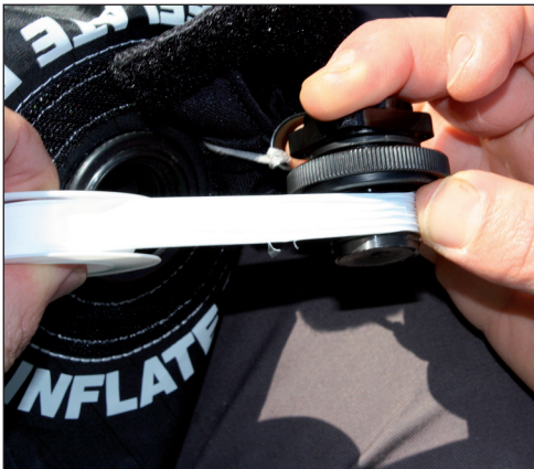
Apply tape to the thread at the base of the inflate/deflate valve
