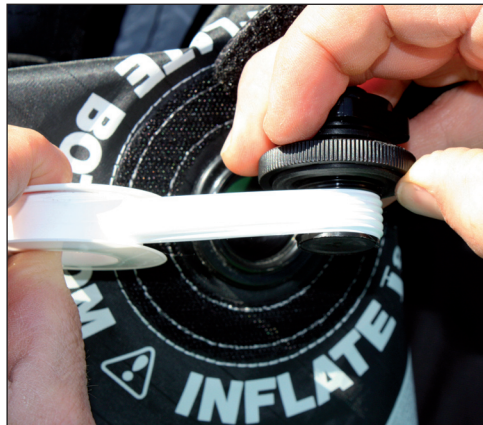
Wrap the tape around the thread four times with tension
